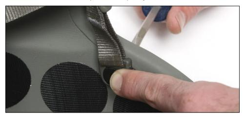
**STEP 2:** Insert another flathead screwdriver into the gap between the webbing and the edge of the T-nut as shown. This will keep the T-nut from rotating while you tighten it the rest of the way in until it is flush in the recess of the plastic anchor.
